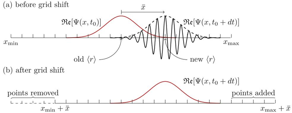
**Figure A1.** Illustration of the moving grid procedure. The propagation of the wave function  $\Psi(x, t_0)$  for a single time step is shown in (a). The resulting wave function has moved in position and has non-zero momentum. After shifting the grid in coordinate and momentum space, the propagated wave function is now centered on the new grid and has zero momentum (b).
