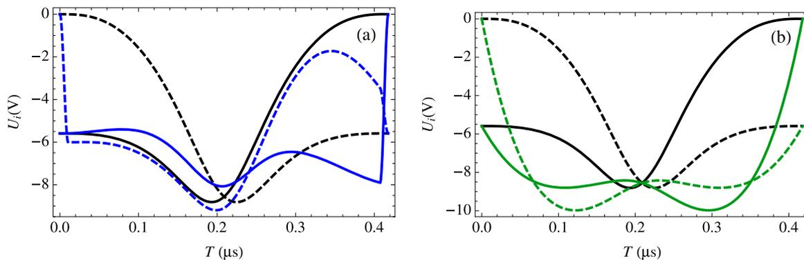
**Figure 2.** Control voltages applied to electrodes for transporting a  $^{40}\text{Ca}^+$  ion from electrode 1 (solid lines) to electrode 2 (dashed lines) within 418 ns for an initial trap frequency of  $\omega = 2\pi \cdot 1.3$  MHz: initial guess voltage ramps (a and b, black) and ramps obtained by classical optimization (a, blue) and the invariant based inverse engineering (b, green).
