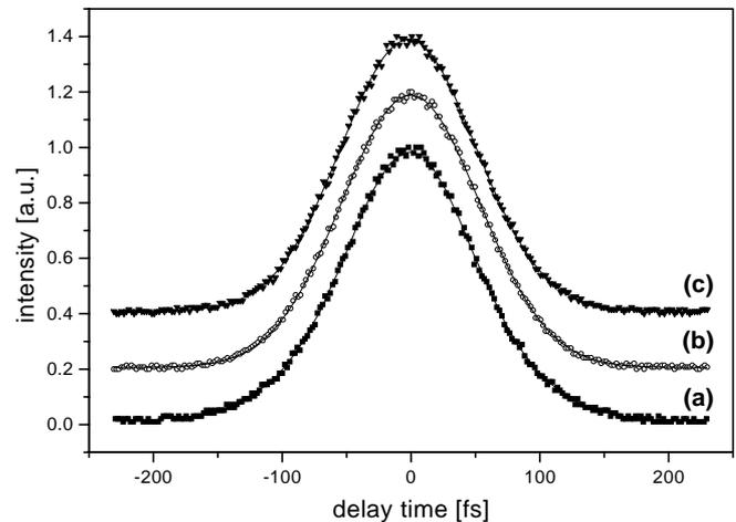
**Fig. 5.** Autocorrelations of unchirped start pulse (a), pulse recompressed by evolutionary algorithm (b), and by “chirp scan method” (c). No difference in pulse length is detectable, which is a sign for the high fidelity of the algorithm-conducted reconstruction
