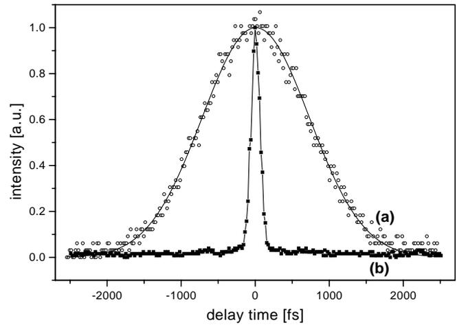
**Fig. 4.** Autocorrelations of broadened input pulse (a), and of recompressed output pulse (b). The evolutionary algorithm automatically finds a display configuration capable of compensating for the chirp introduced by the SF10-rod
