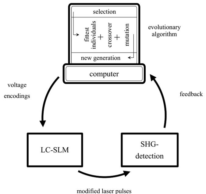
**Fig. 2.** Feedback loop. Given voltage encodings generate specific second harmonic signals. The best patterns are selected and allowed to produce their offspring by mutation and crossover. The new generation is then tested, and so forth
