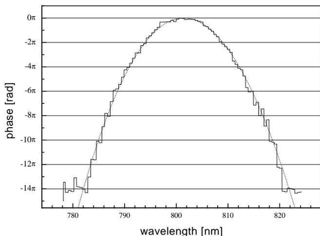
**Fig. 6.** Display introduced phase vs. wavelength (solid curve). The discretization is due to the finite pixel size. The quadratic dependence is characteristic for the second order GVD resulting from propagation in SF10. It is extraordinarily well compensated for by the algorithm, as can be seen by a comparison with the chirp  $-2.59 \times 10^4 \text{ fs}^2$  (dotted curve) obtained from the "chirp scan method"
