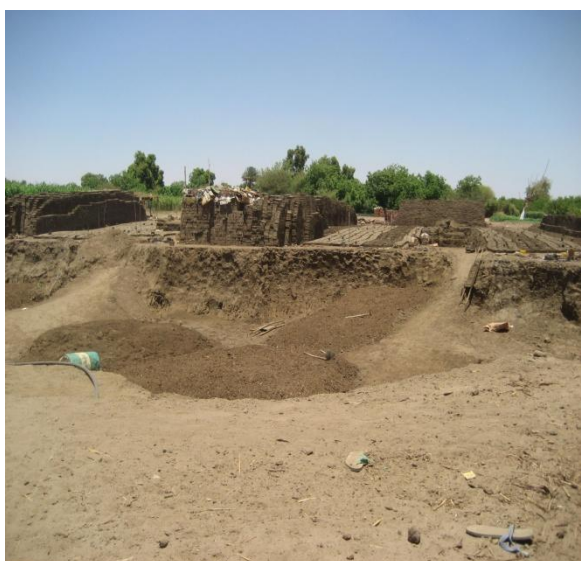
3. Excavation in soil pit for mixing clay and dung
