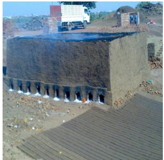
8. Burning of raw bricks in kiln using biomass fuel (fuel wood and compacted dung)
