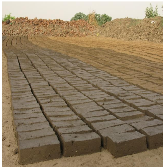
6. Air drying of raw bricks units
