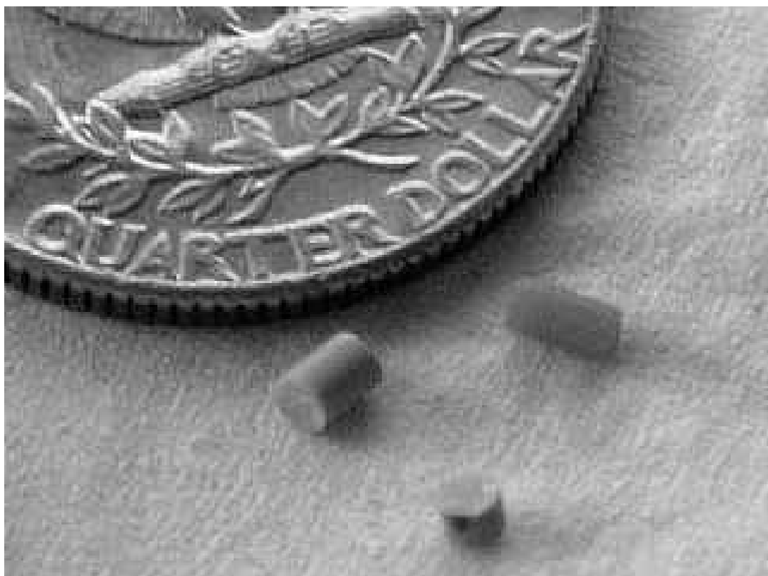
Figure 4.8: Small cylinders of sintered \beta -sialon were used as starting material
