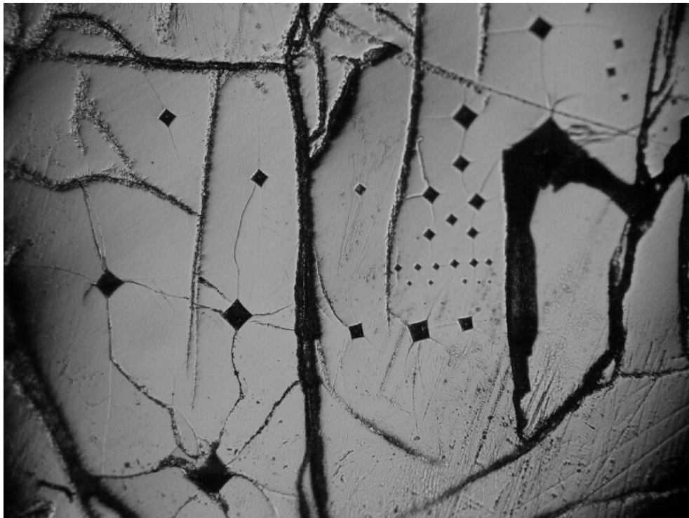
Figure 4.25: Various indentations and extensive cracking in sample HP-Sial22-II
