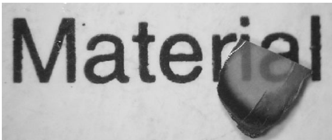
Figure 4.34: A transparent \gamma -sialon platelet from sample HP-Sial40-II. Width: \sim 1 mm
