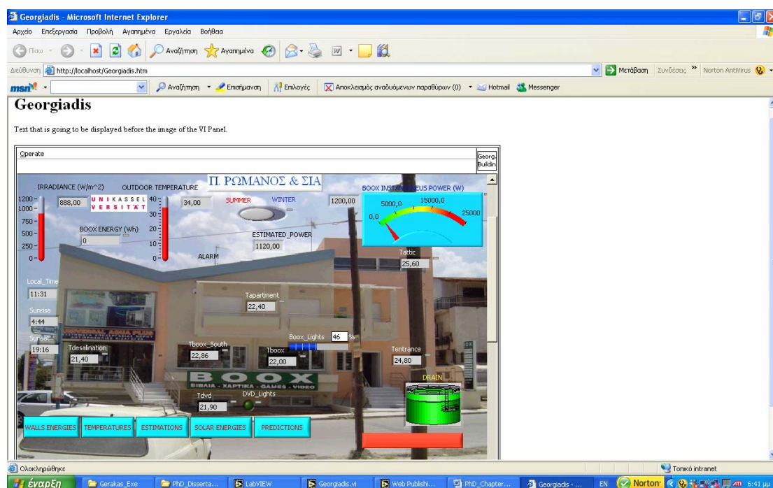
Figure 2.17: Remote Web Panel of the SCADA.
