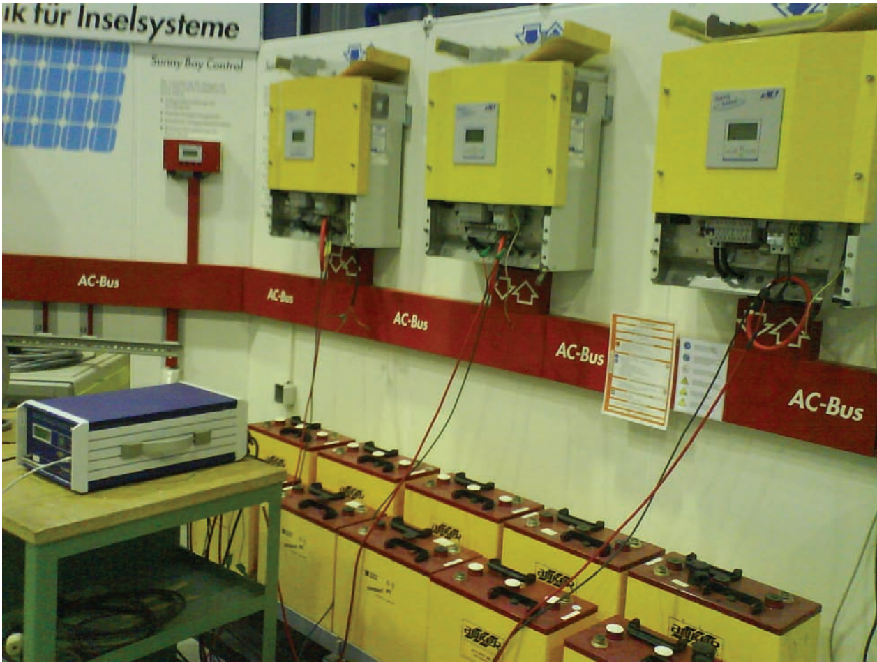
Figure 4-4: Three phase Sunny Island 4500 battery inverter cluster with connected Haag measurement devices [Photo by author]
