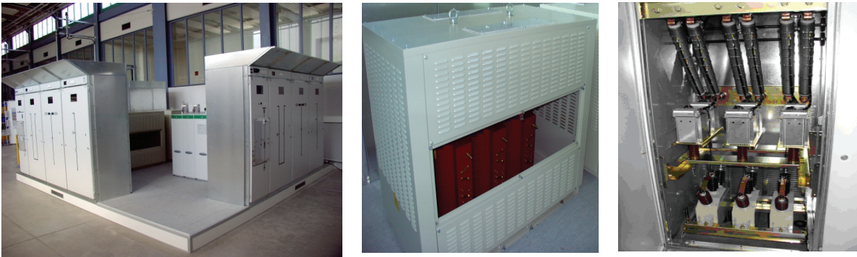
Figure 4-2: General view of Hardware Network Simulator(left), one of the transformers in security cage (middle) and a view of transmission line (consisting of configurable R,L,C elements) [35]
