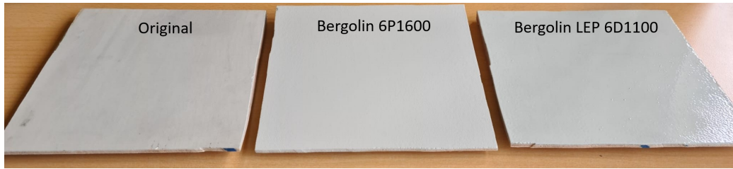
Figure 6. Rotor blade sections with different coatings. On the left is a section with the original coating dating from 22 years ago, in the middle one with the Bergolin coating 6P1600 and on the right one with the Bergolin coating LEP 6D1100. The color RAL 7035 was used for both Bergolin coatings.
