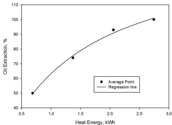
**Figure.2 Essential oil extracted against heat energy required**
