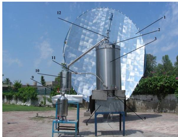
**Figure: 1 A complete solar distillation system**
