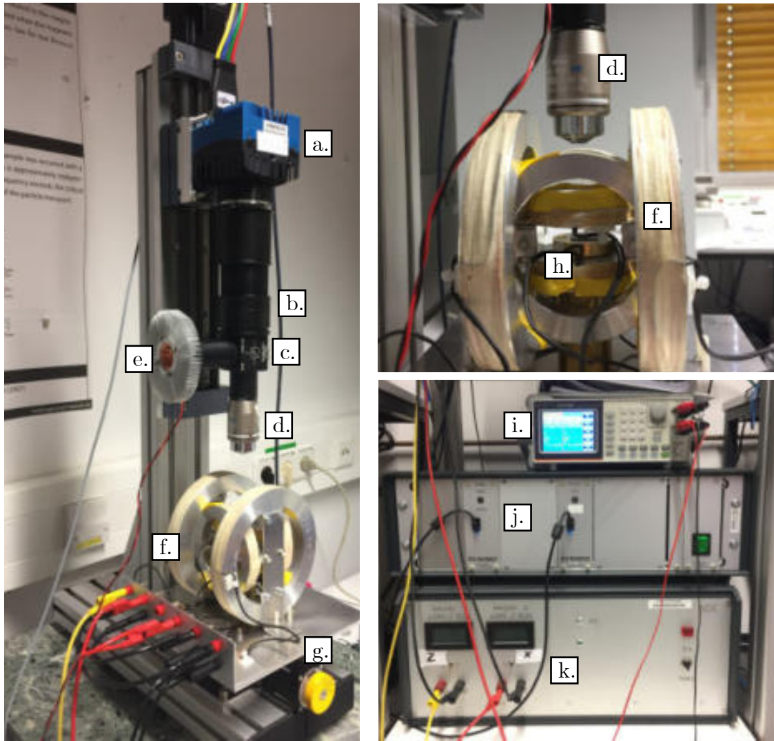
Figure 4.7: Photographs of the rotation / transport setup with the individual components. The optical path (a.-e.), the sample stage (f.-h.) and the electronic control units (i.-k.) are depicted: a. high speed camera, b. tube lens, c. beam splitter, d. 100x objective and e. LED. f. three Helmholtz coil pairs, g. movable stage, h. sample holder, i. arbitrary function generator, j. step motor control unit and k. power supply for two of the Helmholtz coil pairs.
