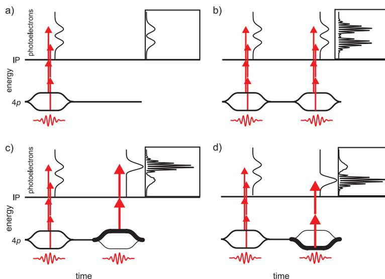
**Figure 4.** Analogy to the double-slit experiment. (a) Two-photon ionization with a single pulse. Photo-ionization with two pulses (b) if both dressed states are equally populated, (c) if the upper dressed state is selectively populated during the second pulse and (d) if the lower dressed state is selectively populated during the second pulse. The insets show the coherent sum of the photoelectron spectra generated during both pulses, i.e. the measurable spectrum.
