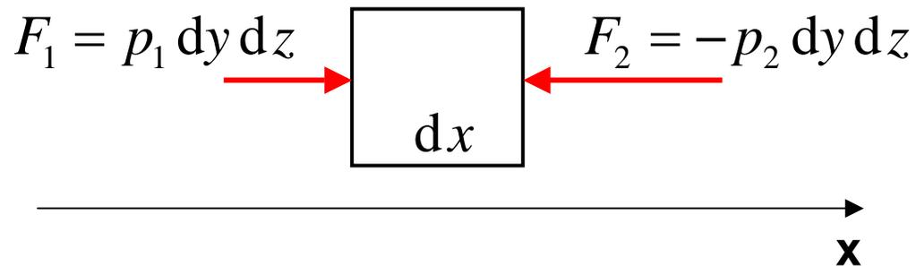
$$F_x = F_1 + F_2 = -(p_2 - p_1) dy dz = -\frac{\partial p}{\partial x} dx dy dz = -\frac{\partial p}{\partial x} dV$$
