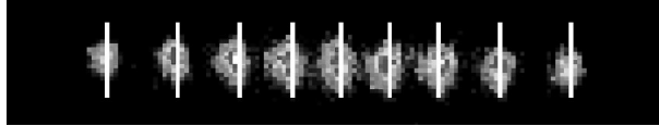
Fig. 3. Ion crystal with automatically determined equilibrium positions. The exposure time \tau was set to 150 ms.
