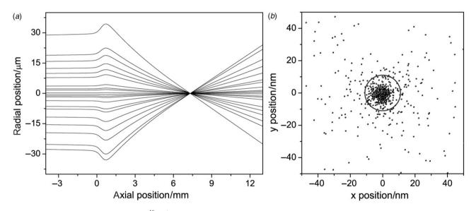
Figure 6. (a) Trajectories of extracted  ${}^{40}Ca^+$  ions at 2 mK which are focused by the lens of Figure 4(c) in the decel-accel mode (65 V) to a 1 $\sigma$ -spot size of 11 nm. (b) Resulting spot diagram in the focal spot around 0.5 mm after the last electrode of the lens (grey circle illustrates the 1 $\sigma$ -spot radius).
