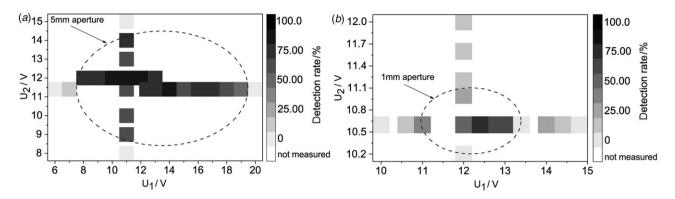
Figure 12. Detection probabilities as a function of the deflection voltages.  $U_1$  and  $U_2$  indicate the potential applied between two opposing blades. The scan clearly shows the edge of the aperture by a sharp decrease of the detection rate. (a) The range can be varied over 10 V and 5 V for the 5 mm aperture. (b) For the 1 mm hole the range where ions can be efficiently detected decreases to 2 and 1 V, respectively.
