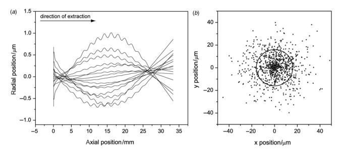
Figure 1. (a) Trajectories of  ${}^{40}Ca^+$  ions during extraction from the trap with an initial temperature of 2 mK. (b) Resulting spot diagram at a distance of 247 mm between trap centre and target amounts to a beam divergence of 134 µrad (grey circle illustrates the 1 $\sigma$ -spot radius of 16 µm).
