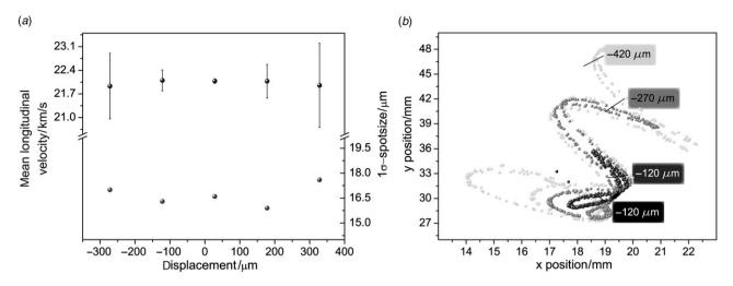
Figure 2. Dependence of the ion beam on the start position (positive values mean towards the extraction direction). (a) Resulting mean longitudinal velocities and  $1\sigma$ -spot sizes after extraction at a distance of 247 mm from the trap centre with deflection electrodes grounded. (b) Resulting spot diagrams of extracted ions when the deflection electrodes are biased to 7.5 V between two opposing trap blades and 9.1 V between the other two blades, respectively.
