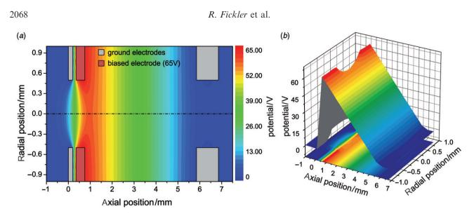
Figure 5. (a) Potential of the lens from Figure 4(c) where the central electrode is biased to 65 V. (b) Three-dimensional view of the potential distribution. (The colour version of this figure is included in the online version of the journal.)
