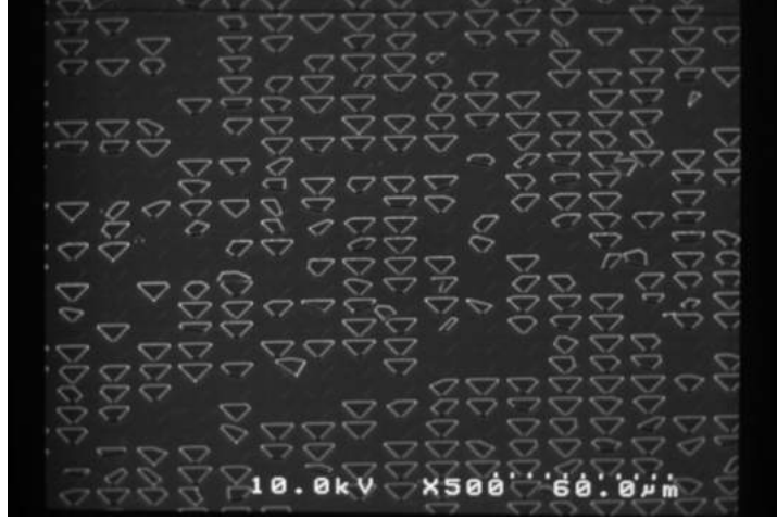
Figure 11: SEM image of the array containing the 10 \mu\text{m} sized structures. Many gaps and structural defects due to complications in fabrication can be observed.
