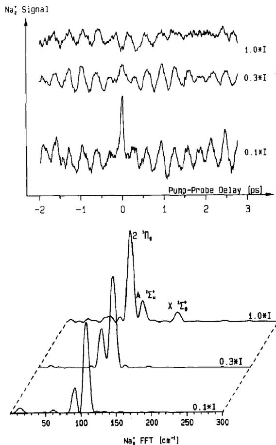
Fig. 2. The upper part of the figure shows transient  $\text{Na}^+$  spectra as a function of delay time between the femtosecond pump and probe pulses. Different intensities were used, as indicated. Below, the Fourier transforms of the transient spectra are displayed.
