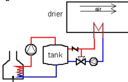
Diagram 2. Heat buffering using a 3-ways valve.
