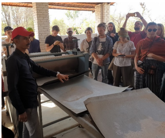
LPPS member demonstrating the flattening of the “desert paper” sheets (Picture by N. El Nagi)
