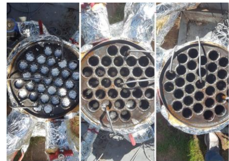
Figure 2: Melting of PCM in Shell and Tube Tank
