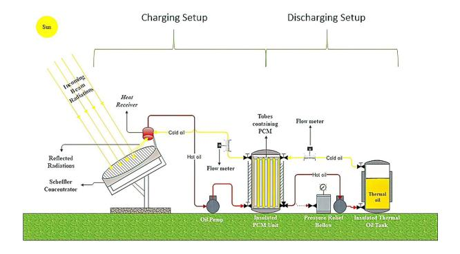
Extensive experimentation during the summer season of 2020-21 shows that the system can store and release 1 kWh and 0.99 kWh of thermal energy with an overall thermal efficiency of 9%. Further investigations are underway to identify the impact of various operating parameters under controlled heating on the performance of the PCM tank as well as on the melting dynamics of the Phase change material.
