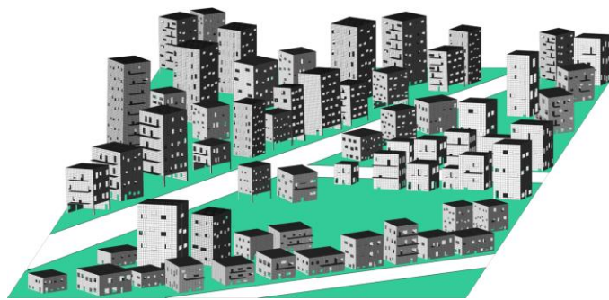
Fig. 3. - A regional portfolio of 3D FE-models for masonry buildings simulated with the SBP-Tool. This can be combined with any seismic input, e.g. wave propagation models
