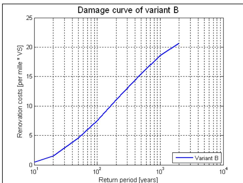
Fig. 6. Damage curve of building variant 2
