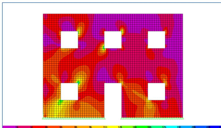
Fig. 8. Example for the principle stresses in a masonry building variant as a result of an earthquake.
