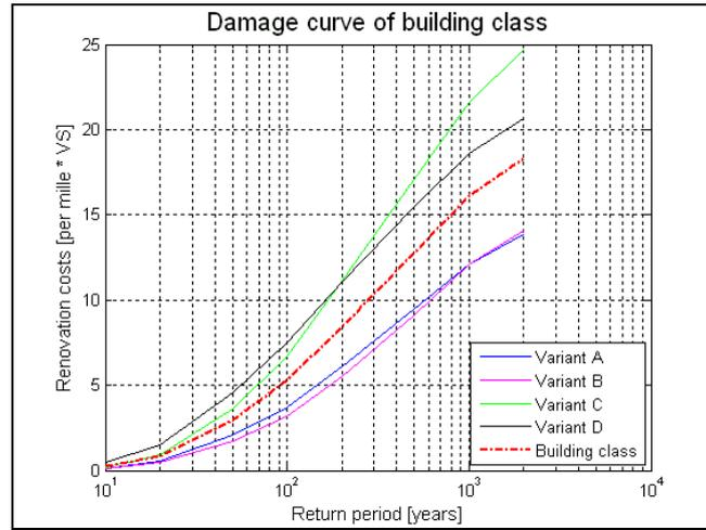
Fig. 9. Damage curves of four building variants for the region of L'Aquila, Italy
