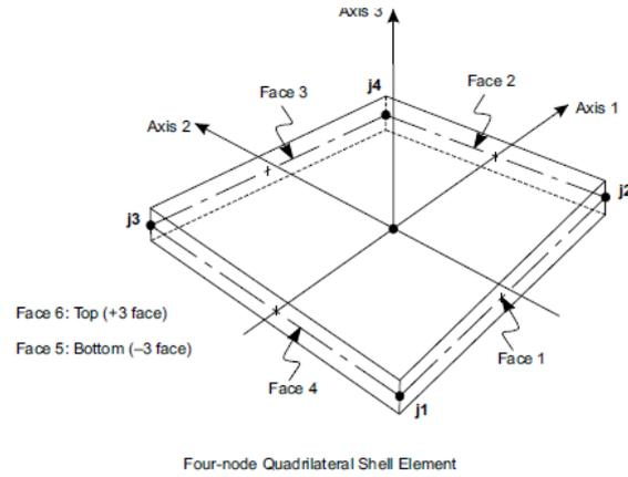
Fig. 5. 3D linear Shell Element (SAP 2000 2008b) used to model the masonry structures in this study
