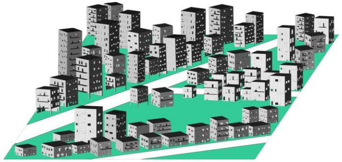
Figure 4. A regional portfolio of 3D FE-models for masonry buildings simulated with the SBP-Tool. This can be combined with any seismic input, e.g. wave propagation models, Mühlhausen (2012b)
