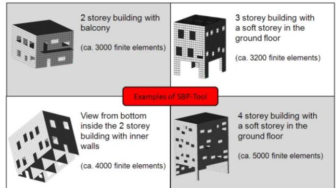
Figure 3. 3D linear FE-models for masonry buildings created by the SBP-Tool, Mühlhausen (2012b)
