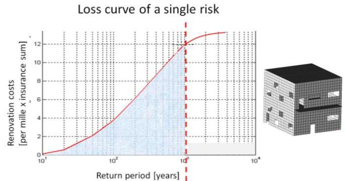
Figure 5. Typical loss curve for one building (right) with the expected linear threshold for masonry buildings, Mühlhausen (2012b)
