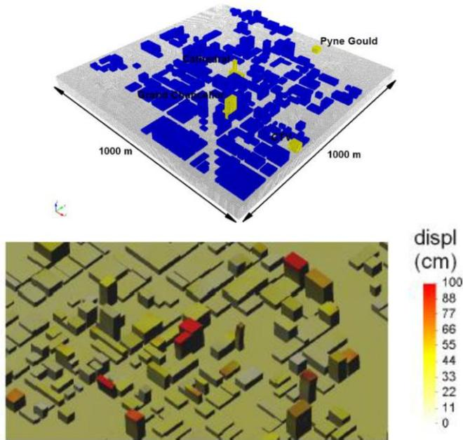
Figure 1. Top: Sophisticated 3D FE model of sub-soil with rigid blocks on top representing buildings in Christchurch. Down: A snapshot of the simulated displacement of the rigid block buildings. Guidotti (2012)
