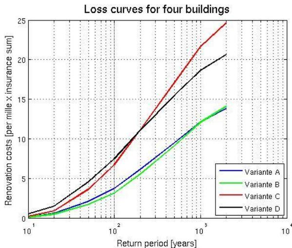
Figure 7. Loss curves for the four buildings from figure 6. Building A,B and C, D may be placed in different loss groups based on their ratio of wall openings, Mühlhausen (2010)
