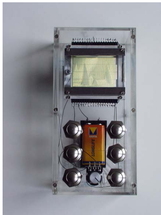
Fig.1: Demonstration box with push buttons and an integrated 3D P-OLED display
