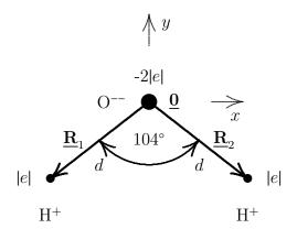
e is the elementary charge (  $e=1,602\cdot 10^{-19}{\rm C}$ ) and d the distance, with  $d=1{\rm nm}$ . Sketch the dipole moment into the figure.
