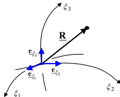
$$\begin{aligned} \xi_1 &= \xi_1(x, y, z) \\ \xi_2 &= \xi_2(x, y, z) \\ \xi_3 &= \xi_3(x, y, z) \end{aligned}$$
