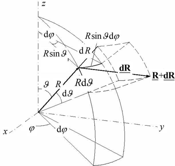
**Metric Coefficients and Vector Differential Line Elements /
