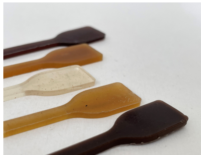
Figure 1: Injection moulded PLA test specimens with chitosan and grape seed extract
