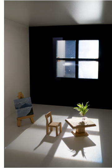
Fig. 4 Demonstrator of a micromirror smart glazing in a dollhouse, visualizing the tailored light guiding and ambience control in a room.
