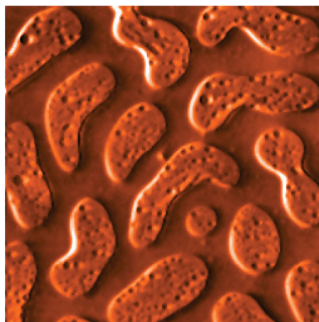
AFM Phase imaging of a SBS (poly(styrene-butadiene-styrene)) and PS (polystyrene) polymer blend sample (Nina Felgen, Technological Physics)
