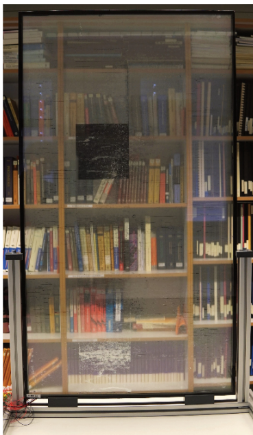
Fig. 2. MEMS micromirror array module housed as double using standard window module manufacturing process, in inert gas environment and sealed with butyl. (a) specially shaped small-scale module closing within 1\mu\text{s} at 80\text{V} for laser safety goggles (b) large-scale module of 71\times 128\text{ cm}^2 closing within 30\mu\text{s} at 70\text{ V} in the center.
