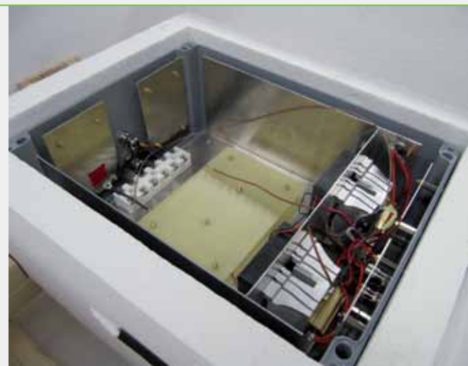
Mess-Kammer des Kalorimeters Test chamber of the calorimeter
