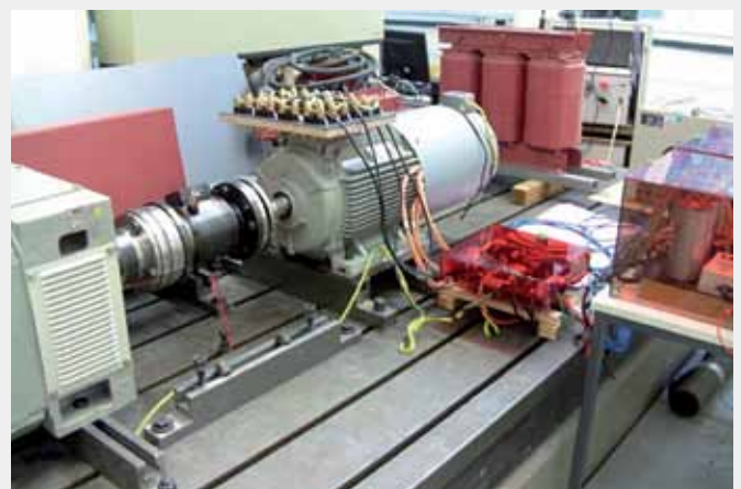
Labor Prüfstand des bürstenlosen, selbst-erregten und -geregelt Synchrongenerators Laboratory test-bench of the brushless self-excited and self-regulated synchronous generator
