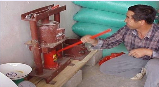
Figure 6. Pressing the blocks with small sized machinery
