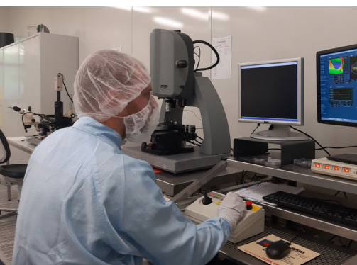
Martin operating the white light interfero- meter in the clean room facilities of the INA
