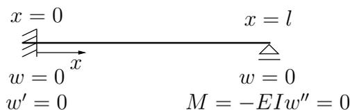
$$EIw''(x) = q_0 \left(\frac{x^2}{2} - \frac{x^3}{6l}\right) + C_1x + C_2 = -M(x)$$
