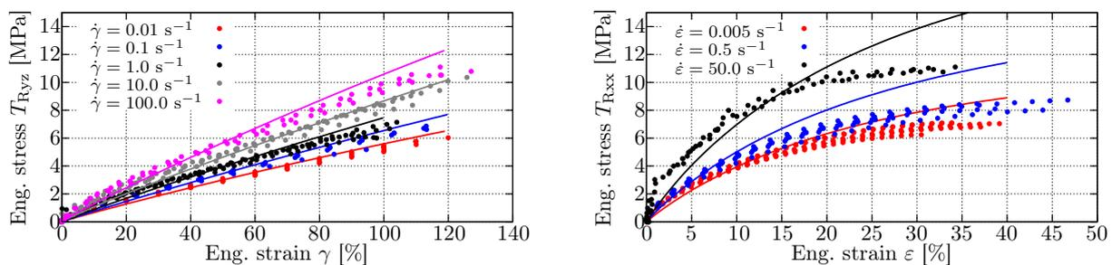
**Fig. 2:** Validation for the TASS (left) and BJS (right) with adhesive layer thickness of 5 mm loaded by different strain rates.
