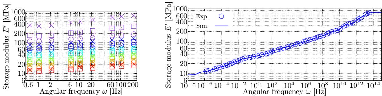
**Fig. 1:** Isothermal curves of the storage modulus  $E'$  (left) from [5], p. 15, and shifted mastercurve (Exp.) with simulation result (Sim.) at room temperature (right).
