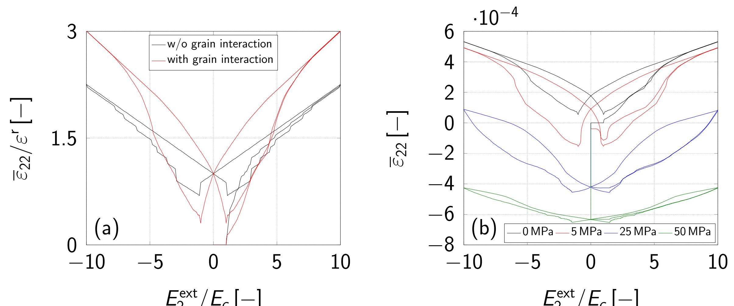
Investigation of the magnetoelectric coupling coefficient  $g_{22}$  of a multiferroic particle composit. Linear (a) and nonlinear (b) material behavior:
