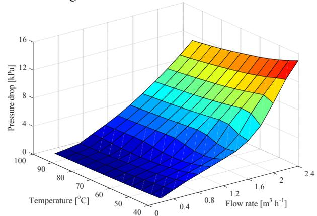
**Figure 4.** Modeled pressure drop of Arcon Sunmark HTHEATstore 35/08 collector as function of temperature and flow rate for 35% propylene glycol/water mixture.
