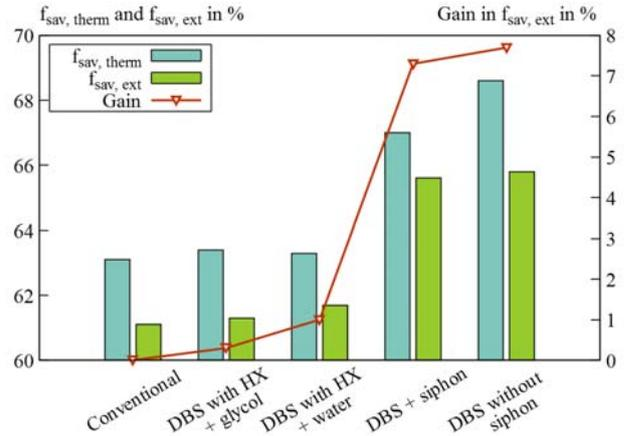
**Figure 9.** Simulated thermal performance during the drying season of a 127 m<sup>2</sup> solar thermal system for drying hay bales using different system configurations.
