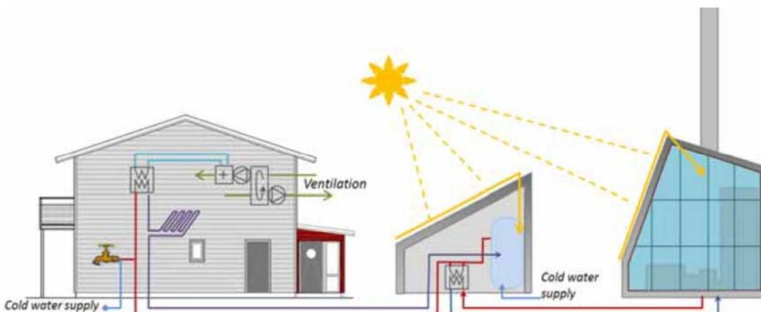
Figure 2: A simplified schematic of the novel heat supply system at Vallda Heberg.
