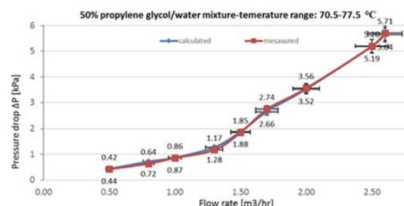
Figure 6. The overall pressure drop of ARCON HT-SA 35/10
