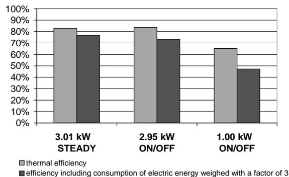
Fig. 5. Thermal and overall efficiency of a 10 kW pellet boiler as measured by [4]. Lowest steady state operation at 3 kW (30% of nominal power).
