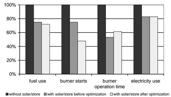
Fig. 7. Comparison of a pellet heating system without solar and two pellet heating system with solar and heat store before [4].
