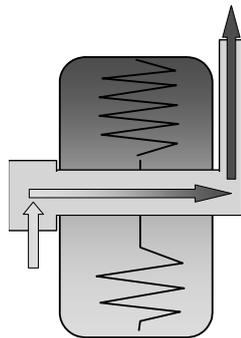
Fig. 3. Buoyancy (natural draft) driven leakage airflow through an integrated burner and its heat exchanger during standby
