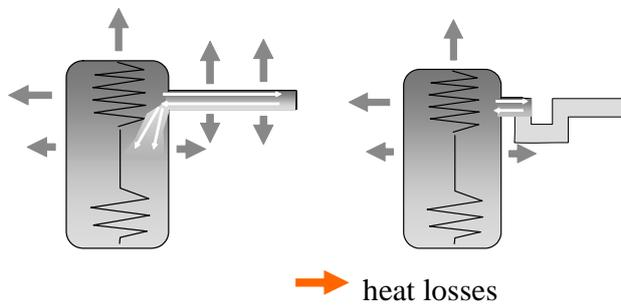
Fig. 8. Pipe connection to store without (left) and with (right) thermosiphon and the corresponding buoyancy driven “in pipe circulation” and heat losses
