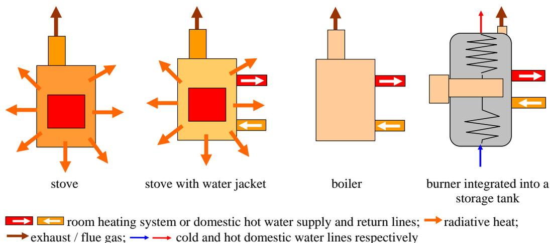
Fig.2. Different types of wood pellet heating systems
