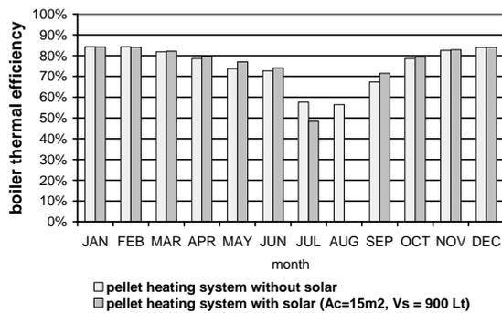
Fig. 6. Pellet boiler efficiency during different seasons of the year, with and without solar system / heat store. In July and August, only very little or no pellet fuel was needed for the system with solar / store. Figure adapted from [4].
