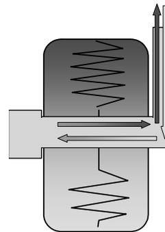
Fig. 4. Cooling out of store by buoyancy driven air circulation without net mass flow / draft through the flue gas heat exchanger of the integrated burner
