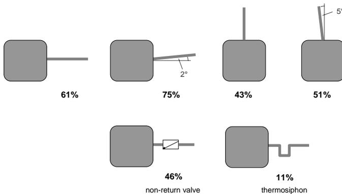
Fig. 9. Measured heat losses of an insulated steel pipe with 2 m length and 1 inch diameter. Heat losses are given in percent of heat losses of the same pipe that would be filled entirely with water at the same temperature as water in the store. Figure adapted from [11].
