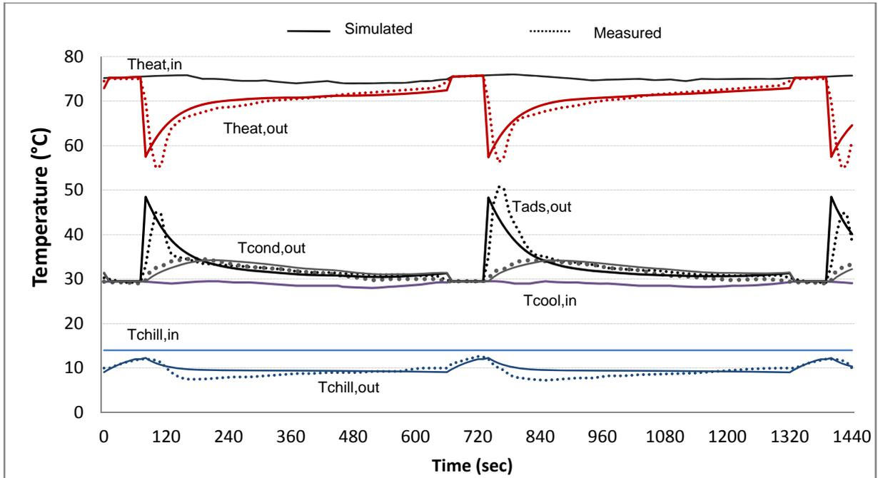
Figure 3: Measured and simulated temperatures of the adsorption chiller (cycle 10 min)
