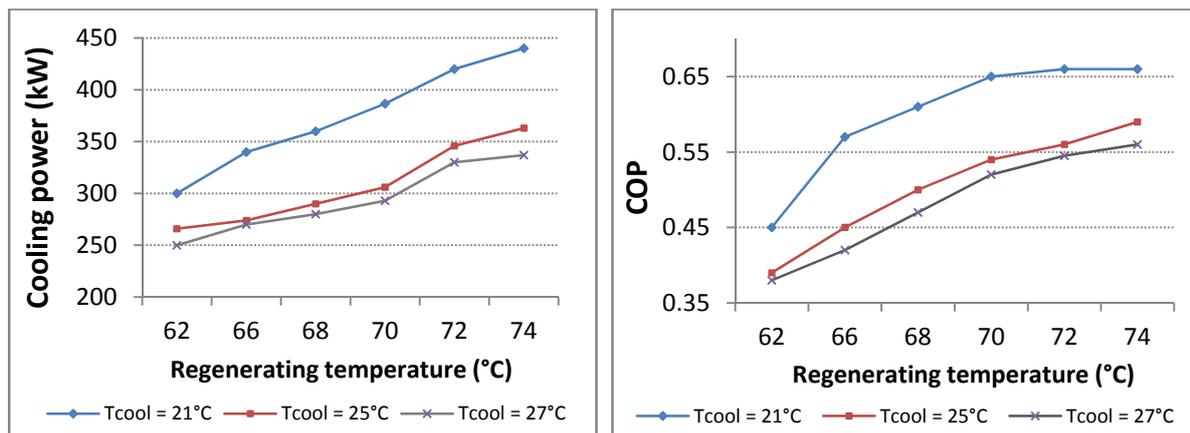
Figure 2: Performance of the chillers (Inlet chilled temperature - 12/13°C)
