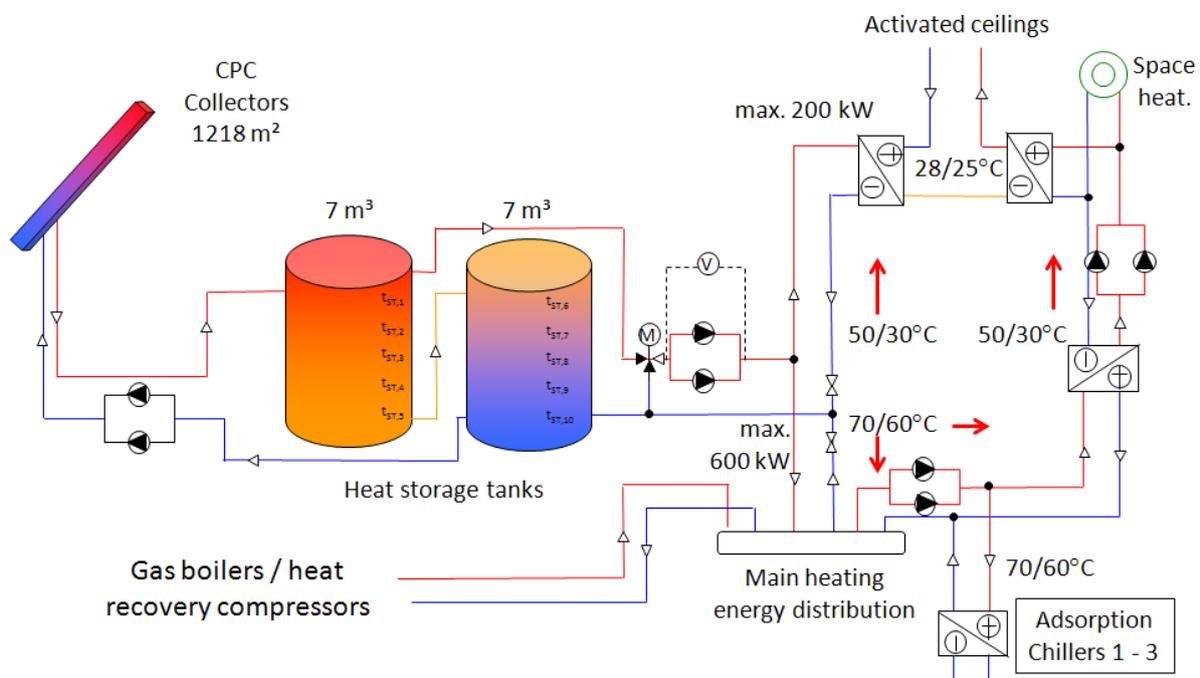
Figure 1: Integration of the solar system in the heating distribution system of the building
