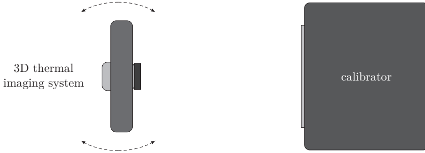
Figure 5.17: Motion of 3D thermal imaging system to calibrate \Delta t_{\text{delay\_avg}} (top view)
