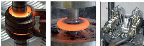
Figure 1.1.: Integrated thermomechanical forming process, cf. (Steinboff et al., 2009)
