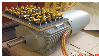
(B) Prototype Synchronous generator 10 kW, 6 poles
