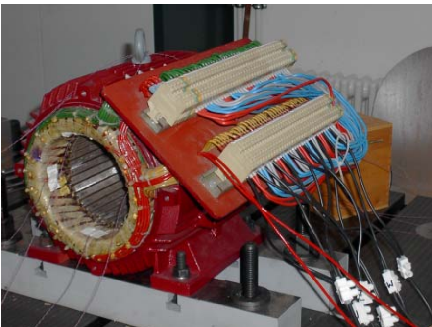
Figure 8.6: Stator part of the test machine showing the installed J-type thermoelements.
