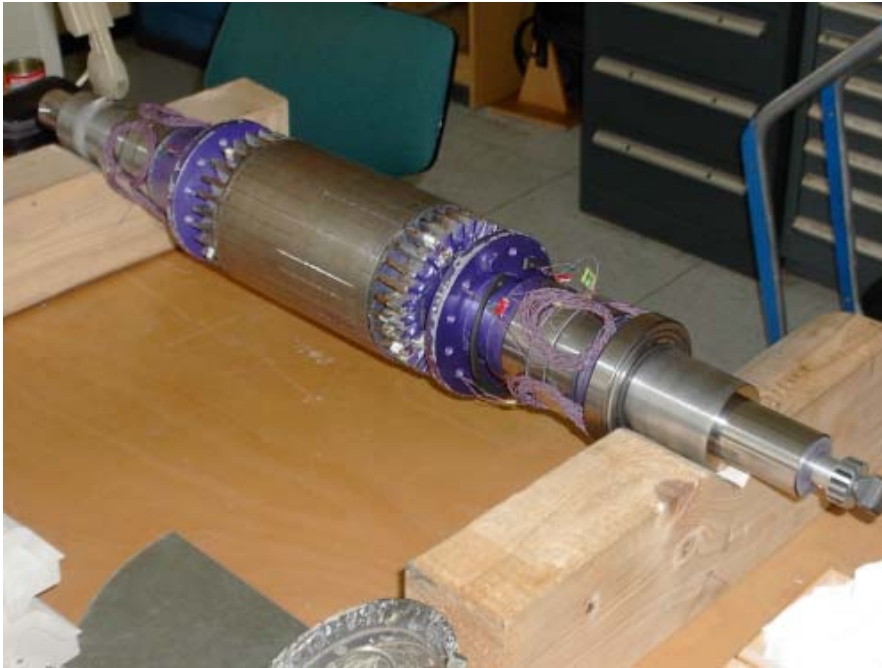
Figure 8.5: Rotor part of the test machine showing the installed J-type thermoelements.
