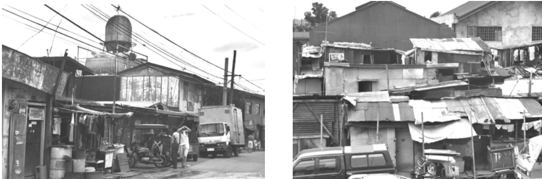
Figure 4q. A high-density residential neighborhood (left) displays a variety of single houses—non-engineered wooden/makeshift, unreinforced masonry, and reinforced concrete structures stand side by side along a road, while informal settlements composed of makeshift, densely packed houses as in the right photo are commonly seen around industrial areas.
