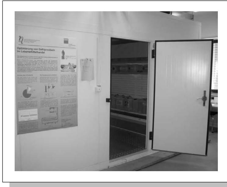
Figure 5.2: Climate chamber for refrigerator measurements
