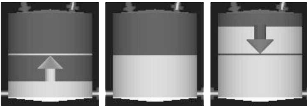
Figure 3: Visualisation of the actual and desired fill-up level ( L ) (left: actual L lower than desired L ; centred: actual L = desired L ; right: actual L higher than desired L )
